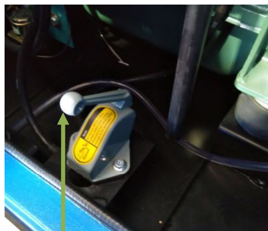
Battery Isolator - ON position
